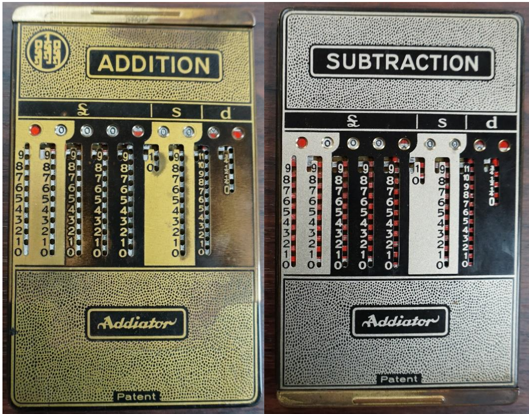
R432 ADDIATOR Basic model SN F976452 F9 means iron cap
